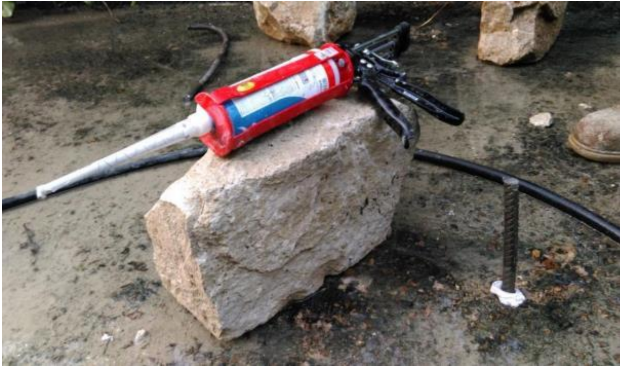
Figure 55: Resin, Purbeck stone and rebar: raw materials for adding roughness to the Hogsmill River in south London: see https://www.southeastrivertrust.org/first-class-degree-in-fish-passage-at-kingston-uni/ for the full case study (Photo: SERT)
